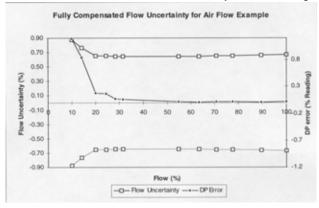
The affect on flow uncertainty from the differential pressure error as flow is reduced is clearly demonstrated by Figure 2. Differential pressure does not significantly affect the flow uncertainty until approximately an 8:1 range down in flow is achieved. Table 2 shows a breakdown of the maximum flow uncertainty. This point occurred at 100:1 range down in differential pressure or 10:1 in flow.
