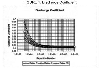
The assumption that the discharge coefficient had a constant value of 0.6 would result in bias errors on the order of 1.5-3.5% for the water flow example and 1% for the gas flow example. These errors can be reduced by calculating a more representative constant discharge coefficient value. In these examples, there are still discharge coefficient variations of up to 2% for the water flow and 0.5% for the air flow which will show up as errors in flow rate.
