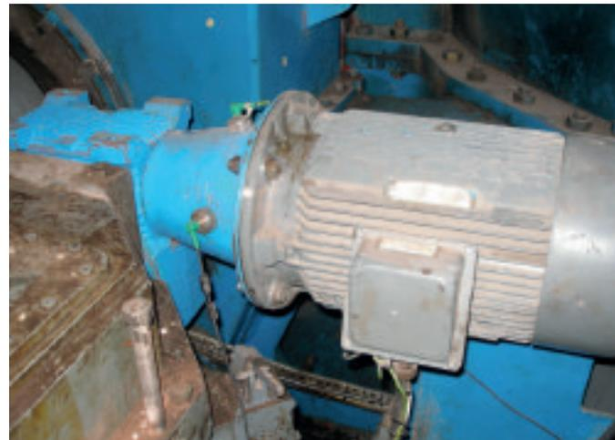
*Vibration sensors attached to a steam turbine barring gear box*
