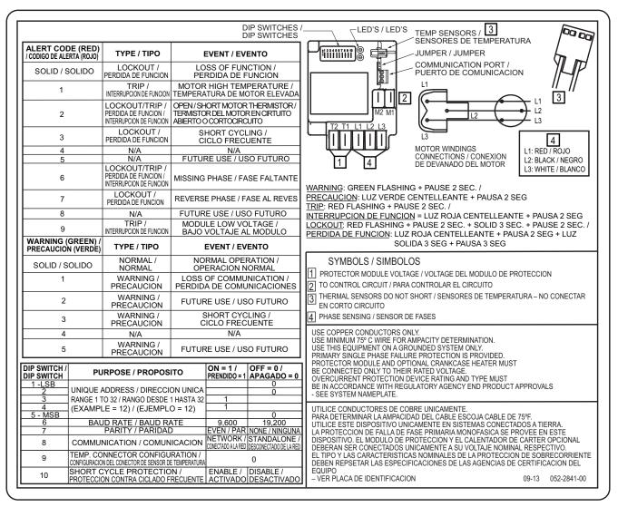
Figure 3 Compressor Terminal Box Wiring with CoreSense Protection
