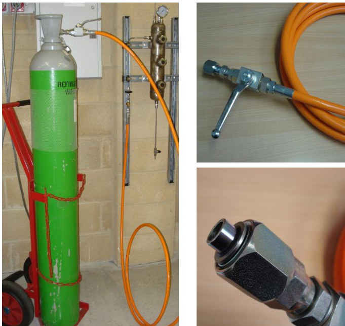
Figure 25. Example of R744 charging equipment
