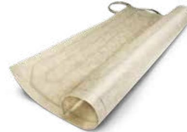
Warm Tiles™ Elite mats are designed for indoor floor warming applications with the least impact on floor height. The WTE mat features a super-thin 0.125 in (3.18 mm) heating mat that conducts heat to the floor surface in the most efficient way. Available in 120 and 240 Vac versions with standard 15 ft (4.57 m) cold leads. Warm Tiles™ Elite mats consist of heating cable interwoven into slim, durable fabric, and come in standard and custom, made-to-order sizes. WTE mats are CSA and UL Approved.
