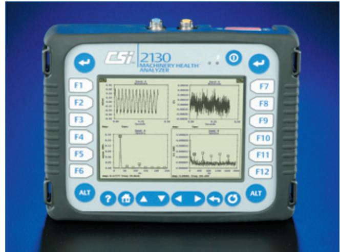
*The full VGA screen displays standard and PeakVue data at the same time. The PeakVue plot (bottom right) provides clear indication of a rolling element bearing fault that is not visible in the standard reading (bottom left).*
