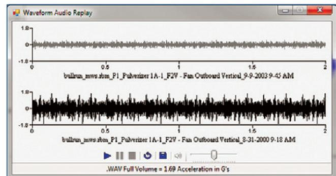
Time waveforms can be replayed from AMS Machinery Manager to listen for machinery defects or for comparison to stored waveforms.
