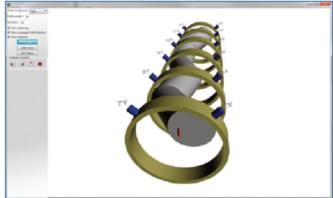
*Use the Live 3D Shaft Animation to see the motion of the shaft around the average bearing shaft centerline. All aspects of the display, including angle of view and playback speed, are controlled by the user.*
