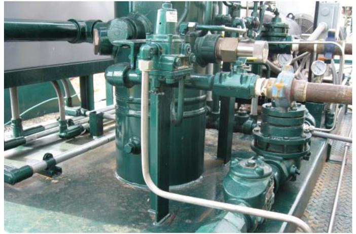
*Producers are looking for low-maintenance, emissions-free solutions for vapor recovery. Copeland Scroll® compressors can take low suction pressure and boost it to 70-275 psig, which gives producers more flexibility to changing field conditions.*
