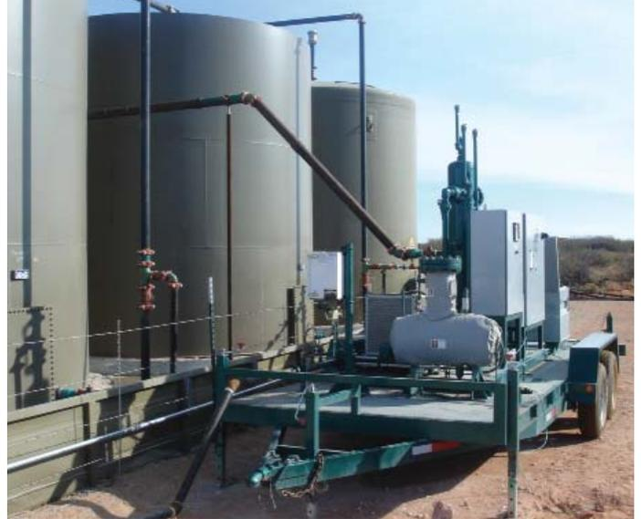
*“The hermetically-sealed Copeland Scroll eliminates the entry of oxygen into the system. Additionally, Scroll offers high runtime efficiency and runs quietly.”*
