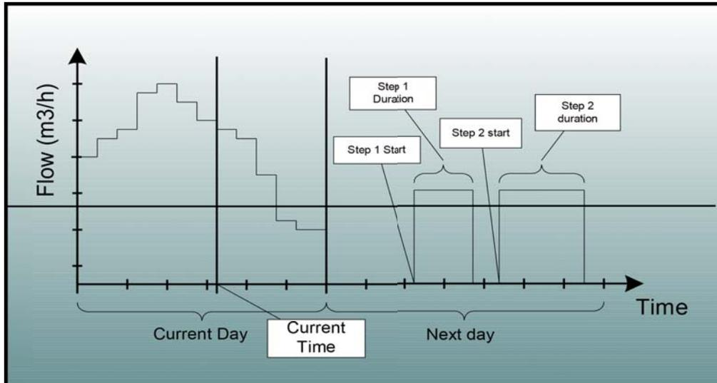
Figure 7. Double Step Flow Curve
