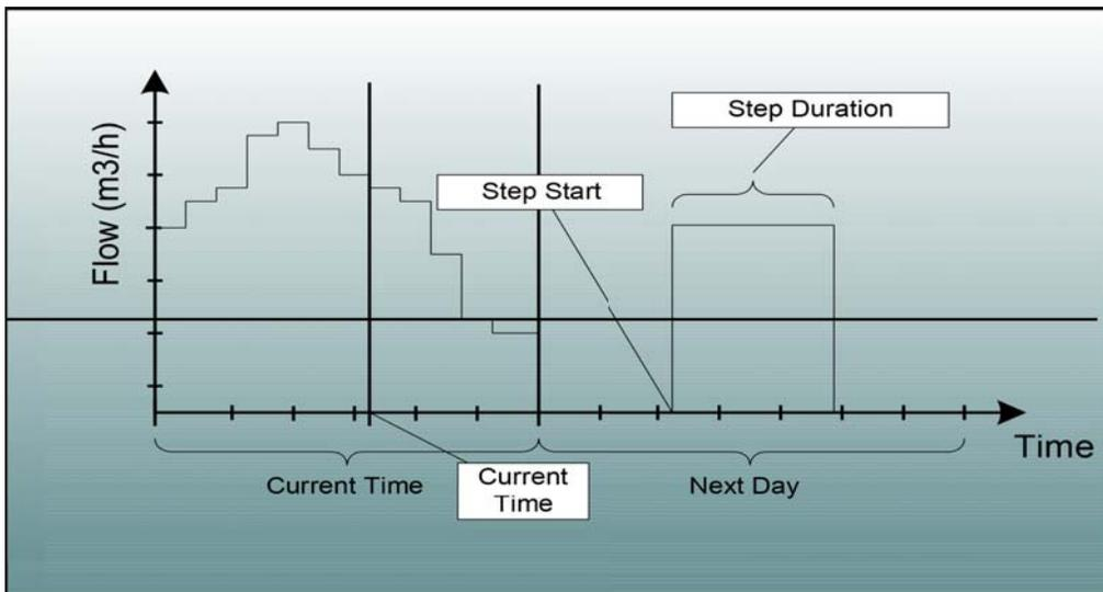
Figure 6. Single Step Flow Curve
