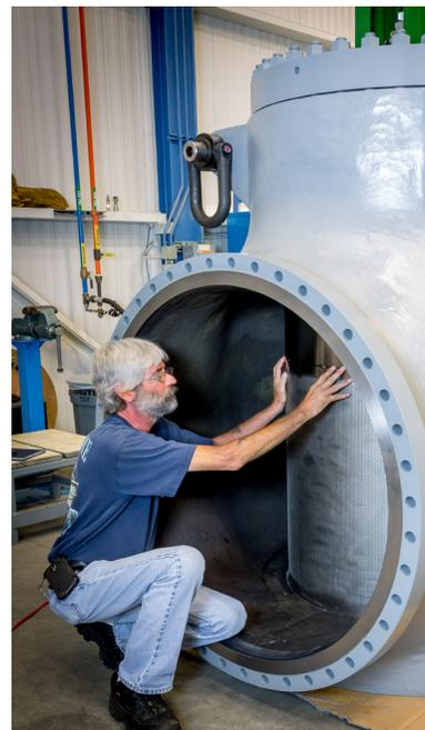
*A customized, drilled-hole cage (inside the body) provides noise abatement on the low end and yet enables the big valve to open under surge conditions.*
