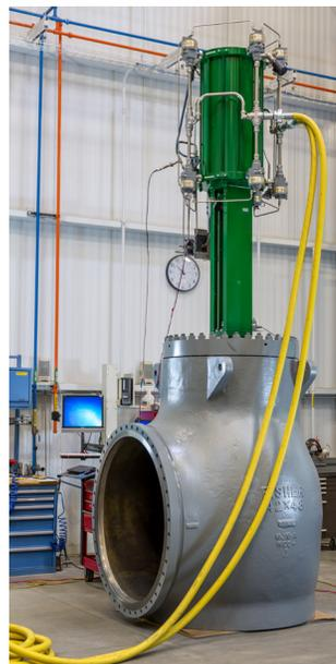
*When completed, the NPS 42x48 Fisher antisurge valve assembly produced in Marshalltown, Iowa, was 15 feet tall and nearly 15,000 pounds.*
