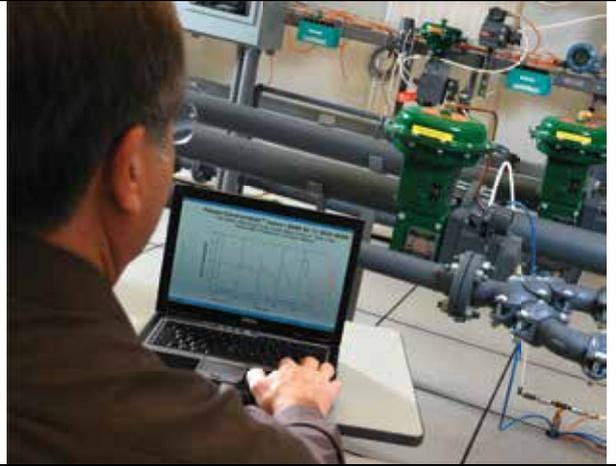
*FIELDVUE™ digital valve controllers (background) provide Advanced Diagnostics to monitor control valve performance.*
