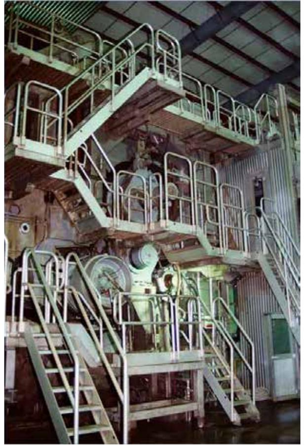
*Pratt installed an OVER Meccanica four-drier type board machine at the Shreveport mill to produce high performance, lightweight linerboard from 100% recycled paper.*
