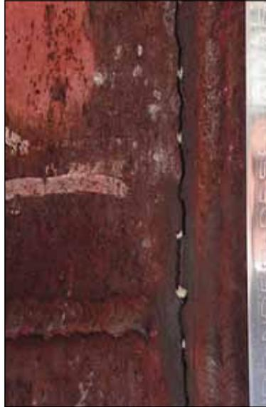
*Cracked steam pipe weld resulting from damaged desuperheater overspray.*
