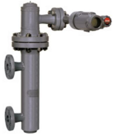
*Fisher caged 249 Series sensors come standard with a liquid damping orifice in the lower equalizing connection that helps stability where vessel capacitance is small and permits narrower proportional valve settings. Displacer reaction to small specific gravity changes allows these instruments to be used in applications where a response to low levels of input signal change is required.*
