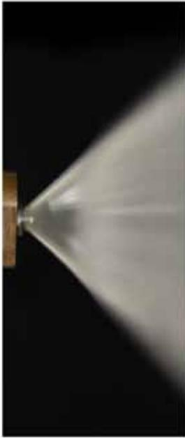
*Clean nozzle allows for proper nozzle spray and water atomization.*
