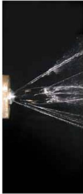
*Clogged nozzle causing distorted spray pattern.*
