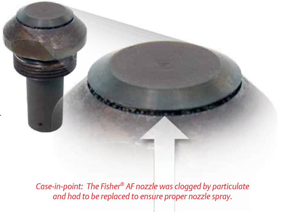
*Case-in-point: The Fisher® AF nozzle was clogged by particulate and had to be replaced to ensure proper nozzle spray.*
