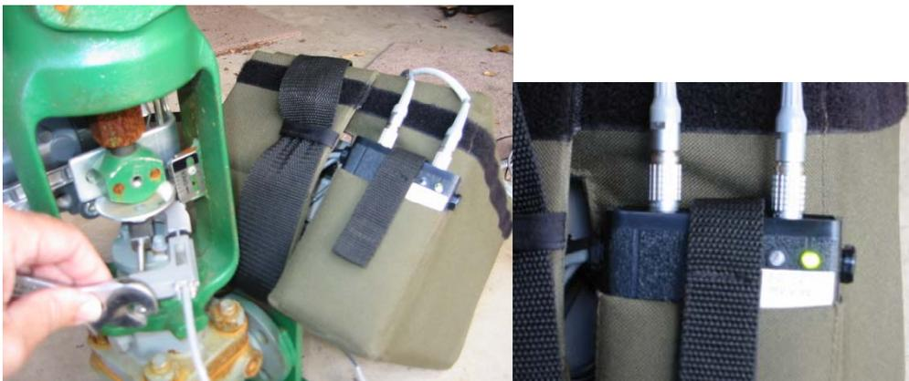
**Figure 4.** Simply adjust c-clamp pre-tension until both LEDs illuminate, and then loosen until one just goes out. No special software or complex procedures are needed.
