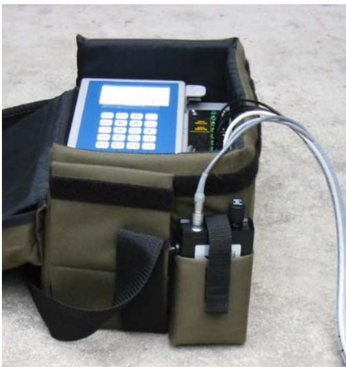
*Figure 1. The FlowScanner 6000 housed in its convenient padded canvas operating bag, with the Interface module integrated into the accessory pocket (left). Shown with cables coiled and ready for transport (below).*
