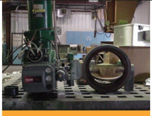
Without a travel deviation alert, this Pf3 RX jacket cooling water valve (NPS8 butterfly) would not have been checked and the metal fragment lodged within it would not have been found. The valve's FIELDVUE digital valve controller alerted operators when it failed to close and avoided a potentially costly delay in the reactor re-start.
