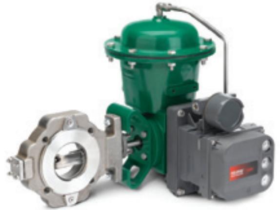
*The Control-Disk™ rotary valve offers excellent throttling performance and an equal percentage flow characteristic, which provides a throttling range comparable to that of a segmented ball valve. This improved capability enables control closer to the target set point, regardless of process disturbances, and reduces process variability.*
