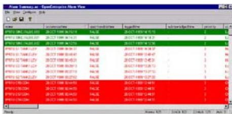
*Alarm client shows all current and unacknowledged alarms in real-time.*
