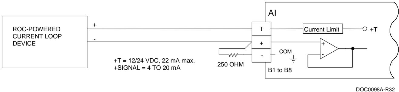
Figure Section: 6-2. Current Signal on Analog Input
