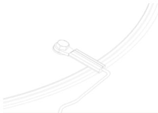
8. Before tightening hex nuts, ensure that the eyelet on the lanyard(s) is pointing **away** from the center of the lid. **Failure to do this may result in damage to the tank** by preventing the unit from opening fully in a pressure event. Tighten each nut to 1 turn after snug.
