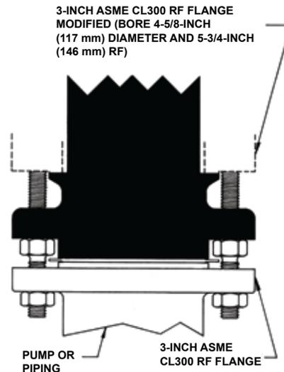
Figure 3. Type C404-24 Typical Valve Installation Schematic
