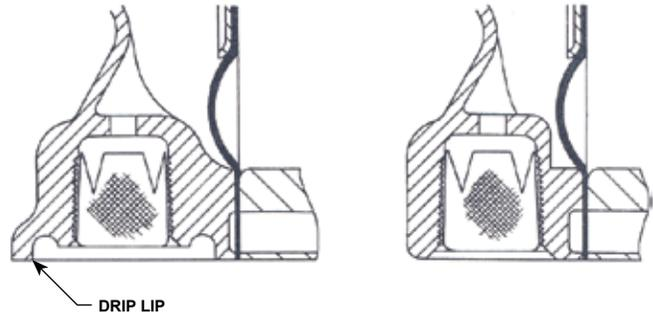
**Figure 1.** Drip lip vent construction has a recessed vent opening while the non-drip lip version on the right does not.
