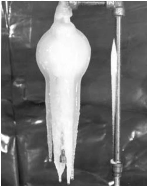
**Figure 2.** Ice completely covered the regulator Fisher Controls used in the freeze tests.
