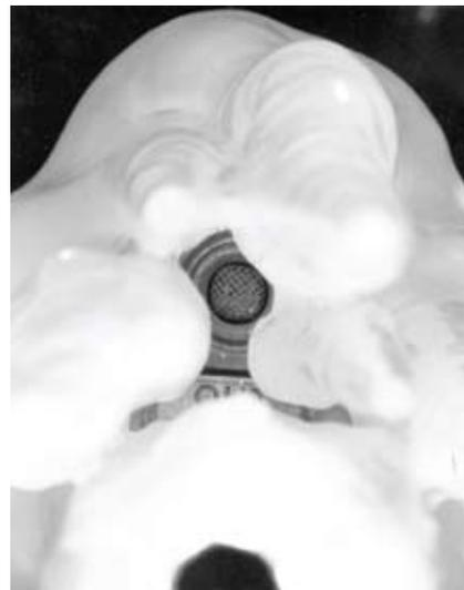
**Figure 3.** Looking up into the vent of the same regulator as shown in figure 2 reveals that the opening remains unplugged.
