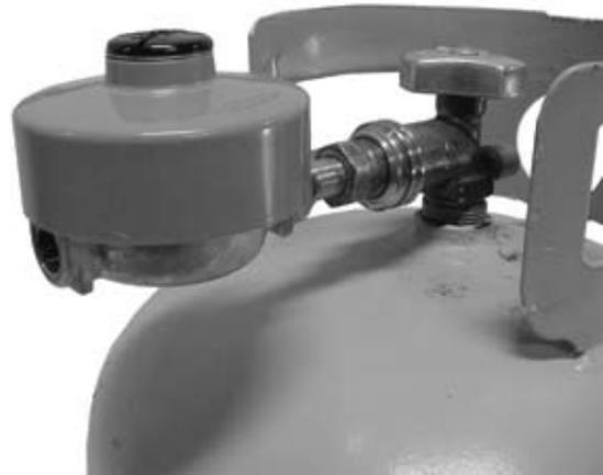
**Figure 7.** Encasements or vent protectors may be able to solve the horizontal mounting problem.
