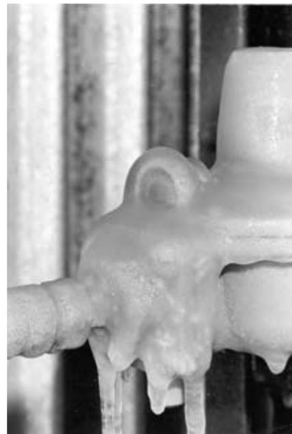
**Figure 4.** Vents on horizontally mounted regulators became quickly plugged during Fisher's tests.
