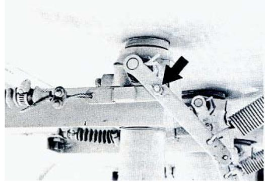
**Figure 3.** To obtain full operating lever travel with some cable controls, the cable has to be attached close to the handle pivot.
