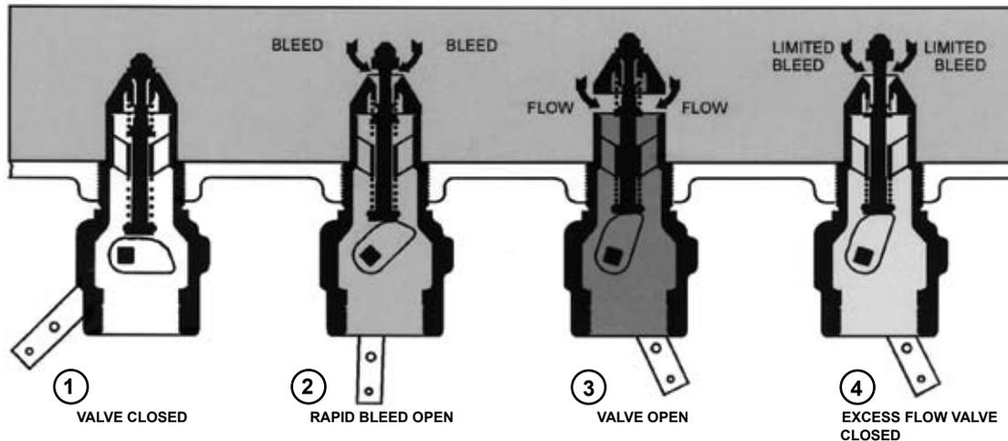
Figure 1. Operational schematic of a typical Fisher internal valve.
