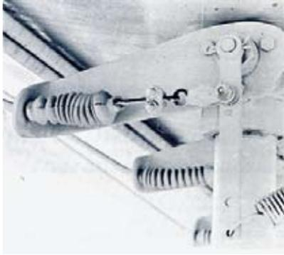
**Figure 4.** The cable should be at a right angle to the operating lever at the mid-travel position.
