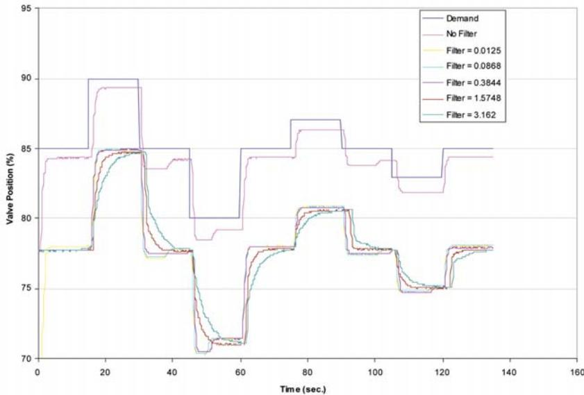
**Figure 2c: Comparison of valve response with tuning set M and various setpoint filter values**
