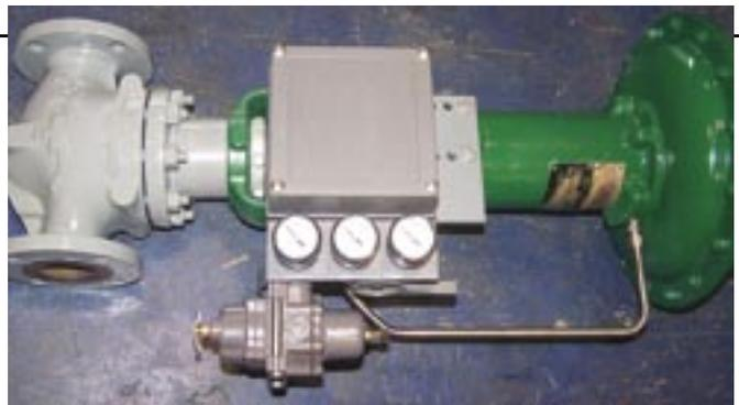
**FIG. 2** Valve/actuator instrument with old nameplate left on after reconditioning and/or repainting.
