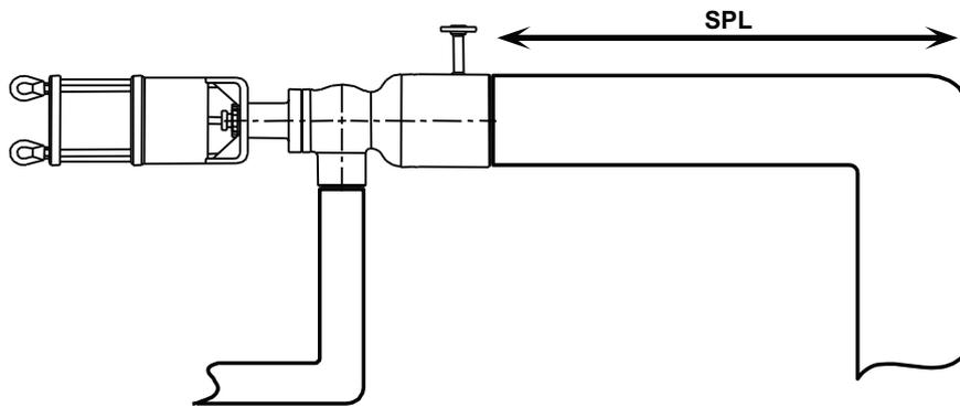
**Figure 5 – Straight Pipe Length (SPL):** assumes 80% vaporization and thermal mixing; calculated by thermodynamics of system; and without obstruction typically over the first 10 to 40 feet.
