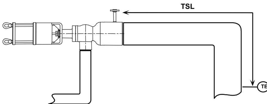
**Figure 6 – Distance to Temperature Sensor (TSL):** assumes complete vaporization and thermal mixing; calculated by thermodynamics of system; and very condition specific—can vary from 40 to 100 feet depending on mass and velocity considerations.
