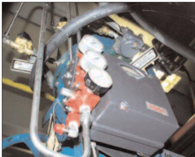
**Figure 2. Original installation with spool valve positioner**
