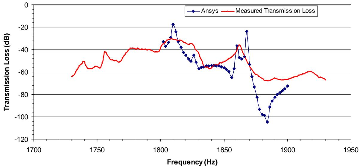
**Figure 11.** Comparison of the measured and calculated transmission loss.
