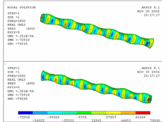
**Figure 9.** Coupled Response at 1802 Hz. (Acoustic resonance frequency)
