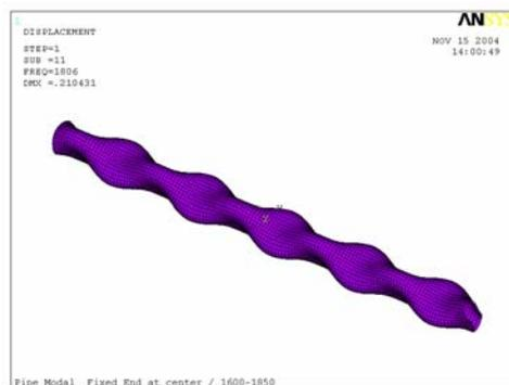
**Figure 3.** Structural Mode (2,11) at 1806 Hz.
