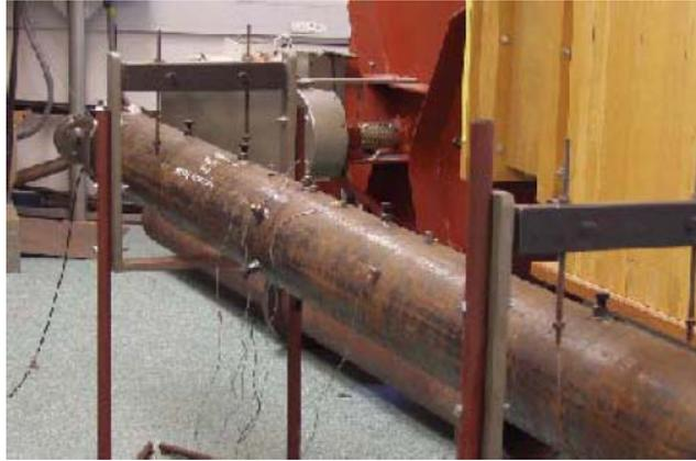
**Figure 1.** Experimental Arrangement (Pipe is closed at left-hand end with loud speaker; pipe is open at the right-hand end (not shown); microphone tappings at several axial and circumferential locations)
