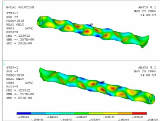
**Figure 8.** Coupled Response at 1818 Hz. (Maximum response frequency)
