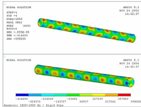
**Figure 5.** Acoustic Mode (1,0,25) at 1802 Hz.
