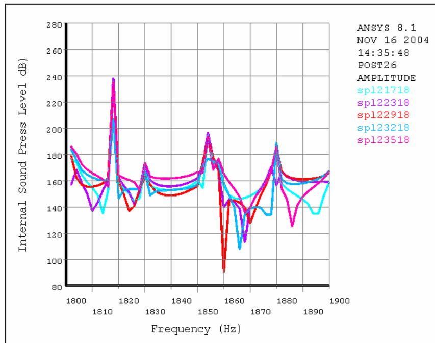
**Figure 7.** Sound Pressure Level versus Frequency for Selected Locations at Inside of Pipe Wall.
