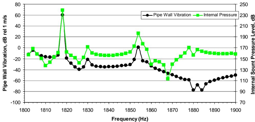
**Figure 10.** FEA calculated sound pressure level and vibration response.
