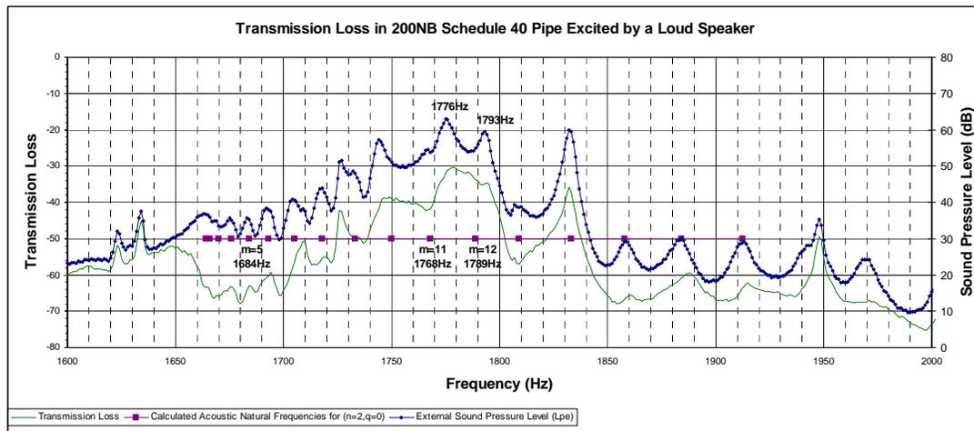
**Figure 2.** Measured pipe-wall transmission loss spectrum at frequencies covering the axial modes  $m=1$  to 18 of circumferential mode  $n=2$ . (Karczub, Fagerlund & Catron[4])
