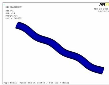
**Figure 4.** Structural Mode (1,6) at 1604 Hz.
