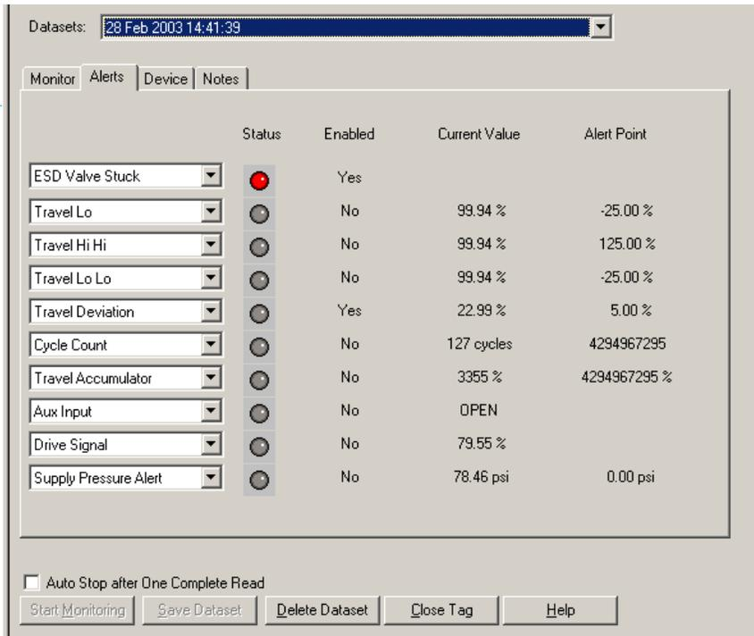
**FIG. 3 – VALVE STUCK ALERT**
