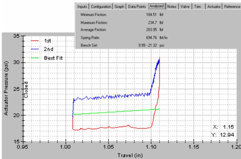
**FIG. 1 – VALVE SIGNATURE TEST AND ANALYSIS ON A SIS VALVE**
