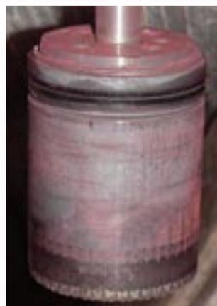
**Gear-tooth damage to feedwater startup valve is attributed to operating at minimum flow for extended periods. Valve plug shown is only six months old**
