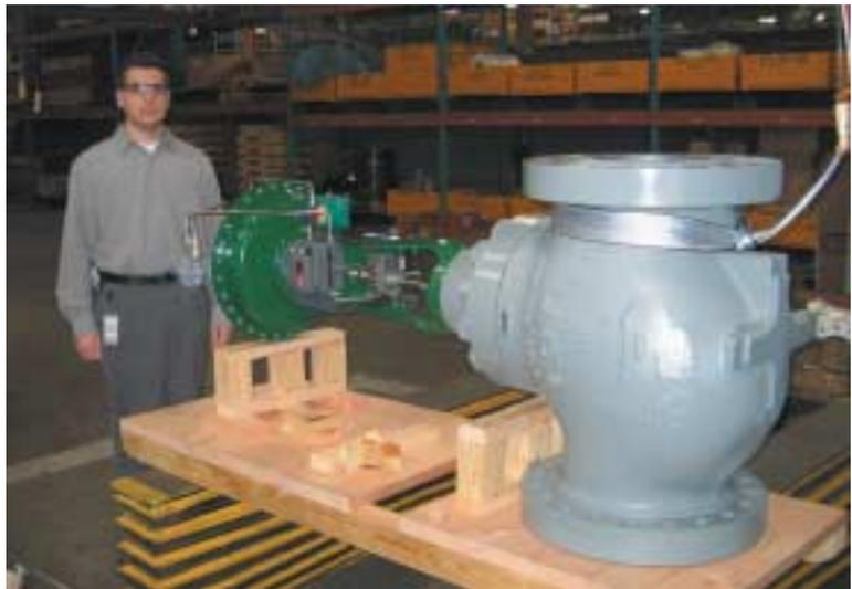
Besides providing the latest in valve-performance monitoring, the Fisher optimized solution also reduces field-tuning time. Traditional antisurge valves require up to 12 hours of in-field tuning to yield desirable results. With the Fisher optimized solution, tuning time is reduced to an average of 30 minutes, without the need for a factory-trained technician. This is possible because Fisher designed the system with accessories that work well together.
