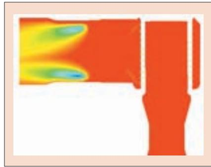
Figure 2: CFD Model of Steam Temperature Profile (left)
