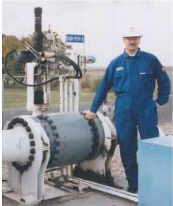
The valve's Hydrodome, seal, and shaft were machined by Fisher Operations personnel in Marshalltown, Iowa. They also assembled and tested the valve to verify its capacity.
