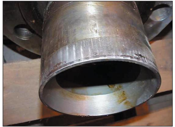
Figure 2. Valve plug damage due to low-lift erosion
