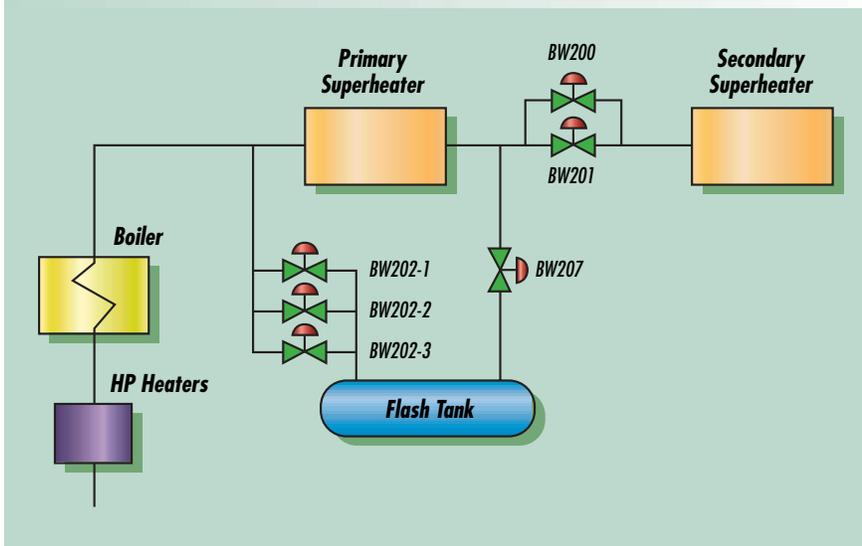
to the flash tank if the operating pressure exceeds 4,250 psig.
