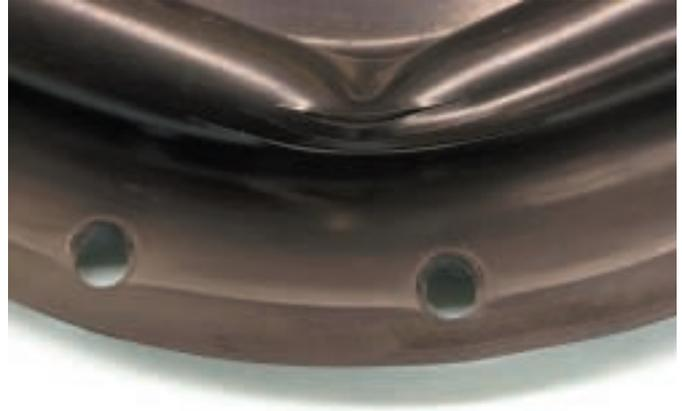
Figure 1: Oxidation cracking typical of exposure to high temperature or extremely long service at normal application temperatures. This is the predominant failure mode of a diaphragm at the extreme limit of polymer aging.
