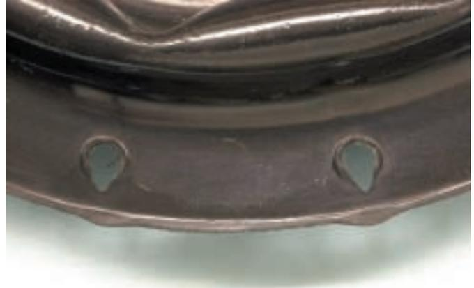
*Figure 3: Typical teardrop shaped bolt holes due to loss of retention (compression set of the diaphragm) and stretching. Notice also the scallop shapes outside each bolt hole and the ledges of displaced rubber both inside and outside the flange.*
