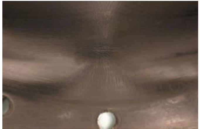
Figure 2: A Nitrile test specimen after 24-hour exposure to 300 ppb ozone. Notice how the crazing is generally normal to the direction of the applied tensile stress imposed by bending. Also, the crazing is so small that it is unnoticeable until the specimen is flexed to open the small cracks. Contrast the size and population of these cracks with the oxidation cracks depicted in Figure 1.
