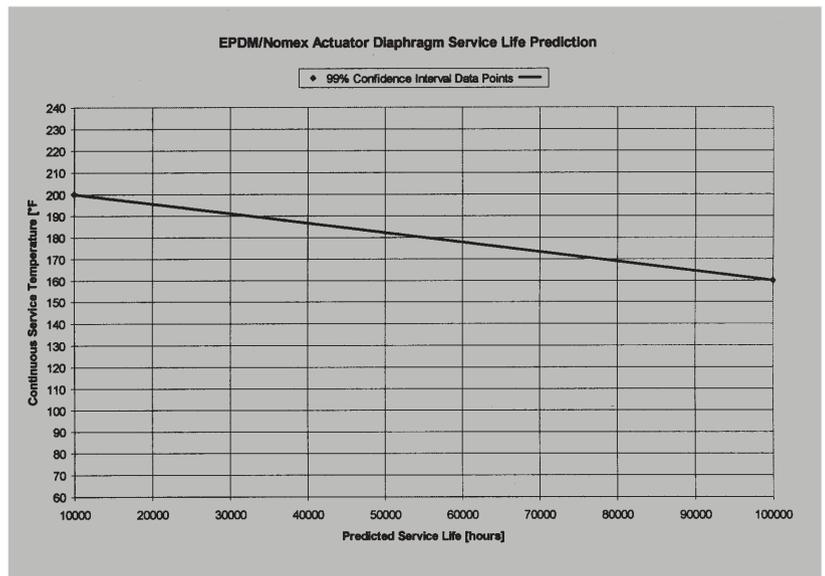
Figure 6. Linear graph that enables the predicting of EPDM/Nomex diaphragm service life. The data presented is based on extensive testing over a four-year period by a major control valve manufacturer.
