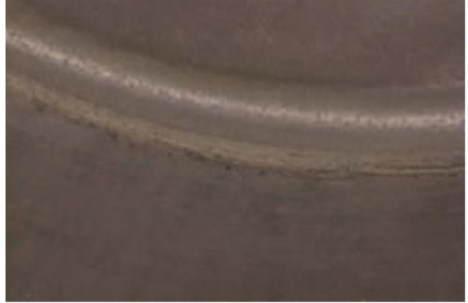
Figure 5: A diaphragm coated with rubber on both sides of the fabric and cycle tested similarly to Figure 4. Even after one million full pressure cycles, only some rubber crumb is visible from abrading the edge of the diaphragm plate, and the fabric is still protected.
