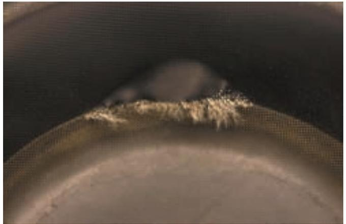
*Figure 4: A one-side-coated diaphragm after cycle testing. Notice that the edge of the diaphragm plate has worn and frayed the fabric until a bursting occurred. This happened after just a few hundred thousand cycles.*
