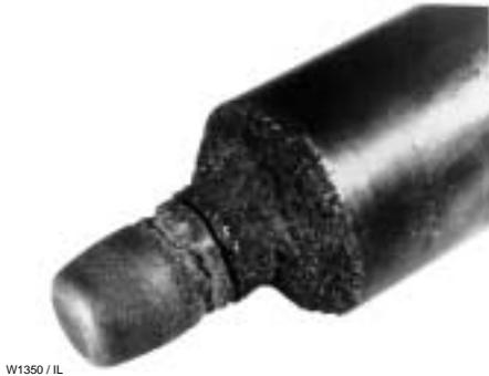
Figure 5. Typical Cavitation Damage
