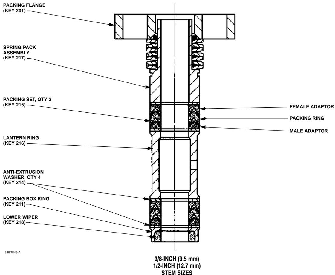
Stems and packing box constructions that do not meet Fisher Controls stem finish specifications, dimensional tolerances, and design specifications, may adversely alter the performance of this packing kit.
