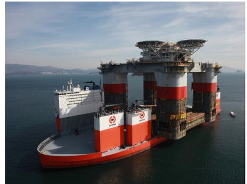
*Dockwise Vanguard is designed for heavy marine transport and offshore dry docking. The length are 275 meter, draft submerged 31,5 meter and max water height above deck is 16 meter. Max lifting capacity 115.000 metric tons.*
