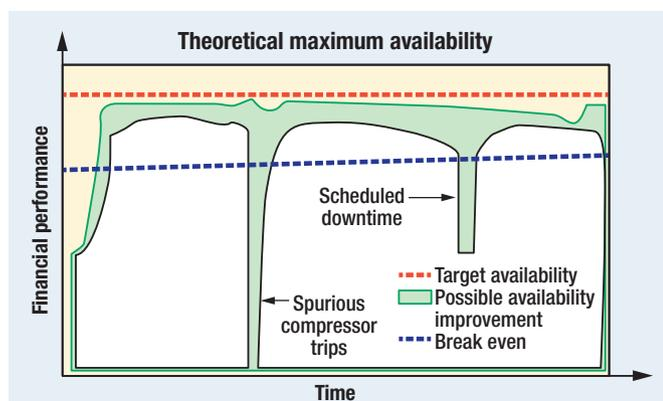
**FIG. 2** Increase compressor uptime by avoiding spurious trips and extending the time between scheduled downtime.
