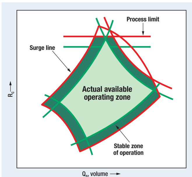
**FIG. 4** Operate confidently close to the compressor's surge line with real-time process and asset data delivered through smart field devices.
