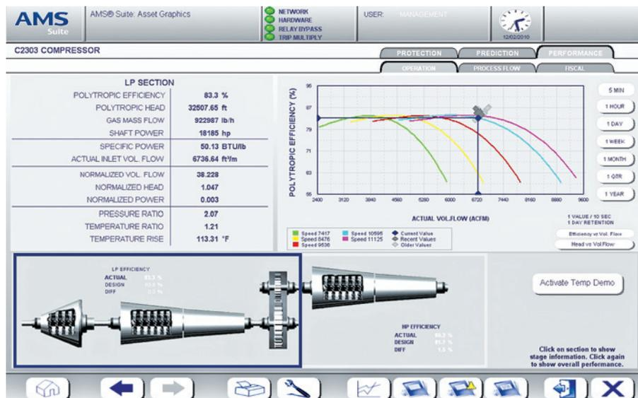
**FIG. 3** The intuitive graphics allow the operator to easily check rotating-equipment efficiency by viewing current process and alarm data along with diagnostic data and any predictions of impending problems.
