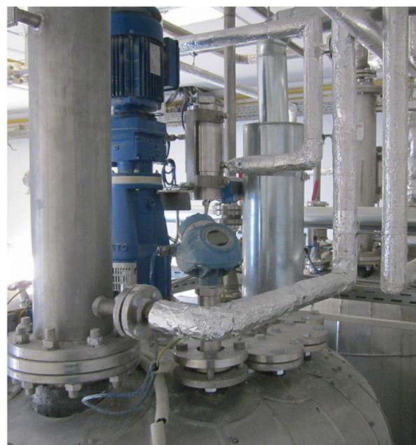
*Rosemount 5402 Non-Contacting Radar with the process seal antenna installed in a 2-in. nozzle allowed for readings despite vapors and condensate.*
