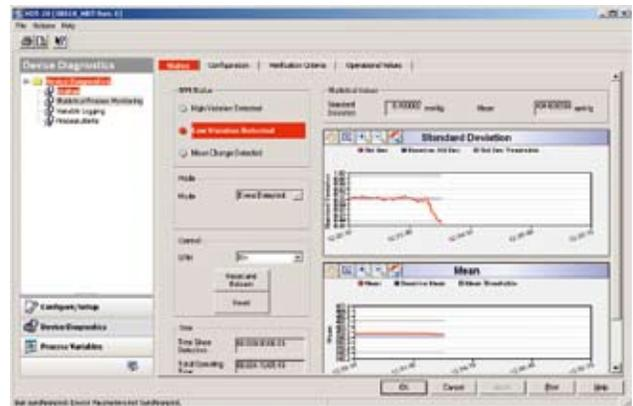
Figure 5: Advanced diagnostics statistical process monitoring.
