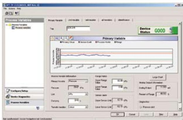
Figure 1: A typical enhanced EDDL process variable screen.
