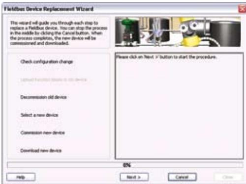
*A software wizard helps to ensure the correct sequence of steps are followed when replacing a device on the fieldbus network.*
