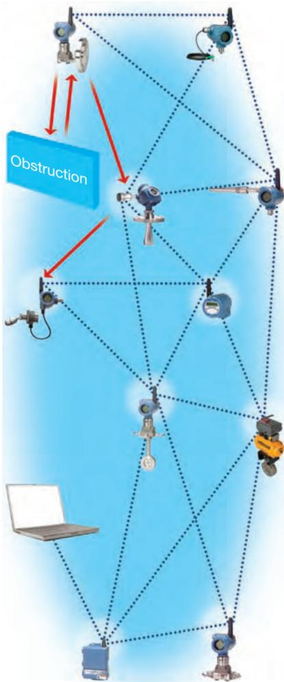
**2. Wireless field networks** based on mesh technology deliver data at greater than 99% network reliability. As new obstacles are encountered in a plant, these dynamic networks can reorganize around them automatically—without any intervention by the user
