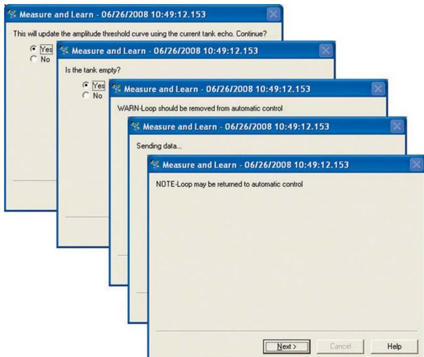
An example of the radar setup wizard based on EDDL 'methods'.
