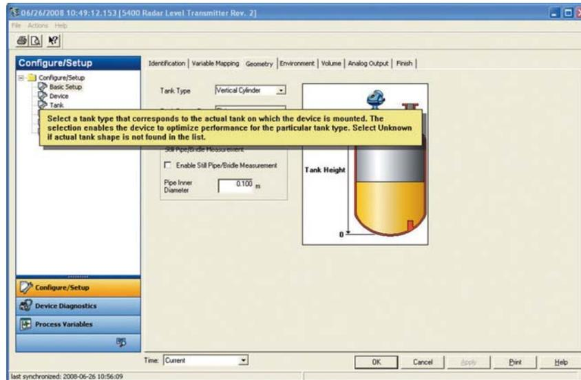
The system provides a help utility which can be used for geometry setup.
