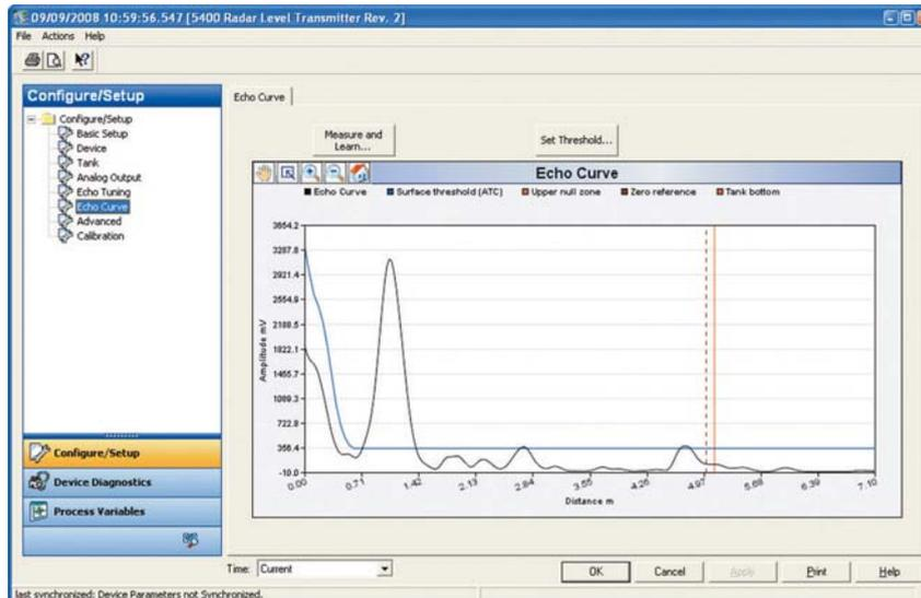
Echo curve and surface threshold waveforms etc. rendered from EDDL graphical elements.
