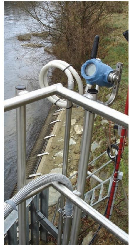
The temperature of the river water is measured using a temperature sensor connected to Emerson's Rosemount Wireless 648 transmitter.
