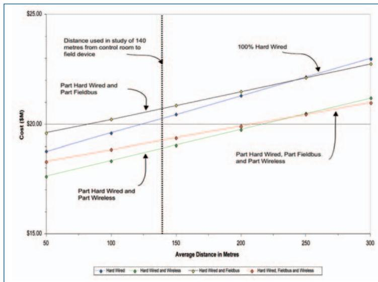
Studies indicate that wireless technology, by itself or in combination with analogous wired technologies, can provide substantial cost savings without increasing risk. (Image courtesy of Emerson Process Management)
