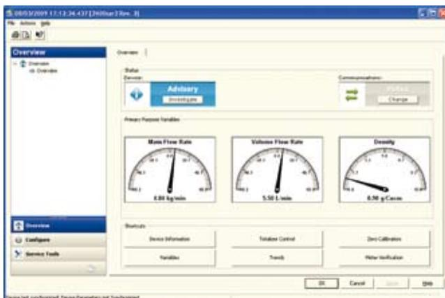
*Through a digital network connection, overall flowmeter status can be monitored without going to the field.*
