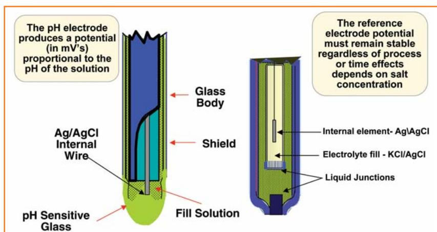
Figure 1: Conventional pH sensor.
