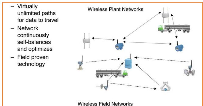
Figure 4: Smart wireless networks based on self-organizing technology.
