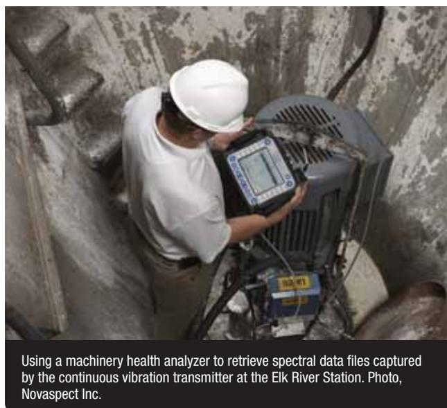
Using a machinery health analyzer to retrieve spectral data files captured by the continuous vibration transmitter at the Elk River Station. Photo, Novaspect Inc.
